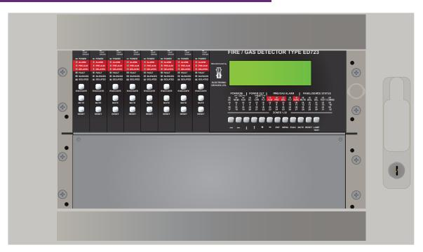
The latest ED700A system provides, in one enclosure, all necessary facilities for Gas and Level Detection. Fail safe operation., Gas and Level modules continue to function after major system failure. Loop communication or microprocessor failure still allow any Discovery or E.D Gas detector to provide alarm indication. The ED700A panel can accommodate up to eight loop modules of ED726 Gas and/or Level Detection giving a total of 80 addressable gas sensors.
